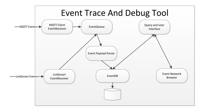
Figure 5: Inner architecture of the ETDT
