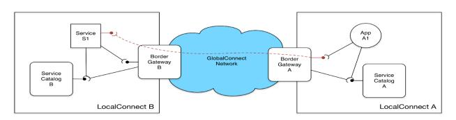
Service S1 in LocalConnect environment B uses the Tunneling Service (REST endpoint discovered in the local Service Catalog) provided by the Border Gateway B (BG B) to be tunneled beyond its LocalConnect environment.
