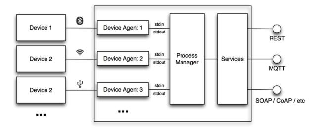
The core of the system is the Process Manager that reads devices/resources configuration and executes corresponding device agents and redirects the system streams
