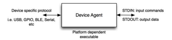
The right side of it describes how the Device Agent communicates with the DGW managing its execution: it is done using the most universal and ubiquitous interface - standard system input and output streams (stdin, stdout correspondingly). The standard system error stream (stderr) is used for logging purposes (data written into stderr will be forwarded to DGW for output in the debug console).
