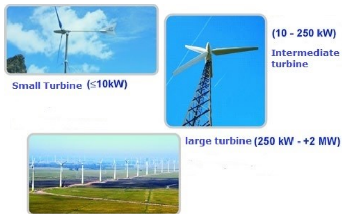
Figure 4 – Types of wind generators 2
